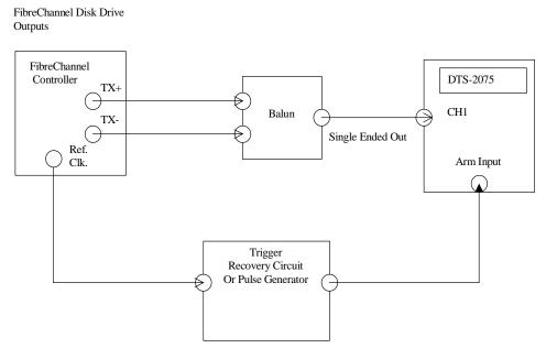
**Figure 1 - Instrument Setup**
